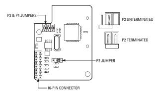
Figure 18. TXB-V Termination and Baud Rate (Bottom View)
